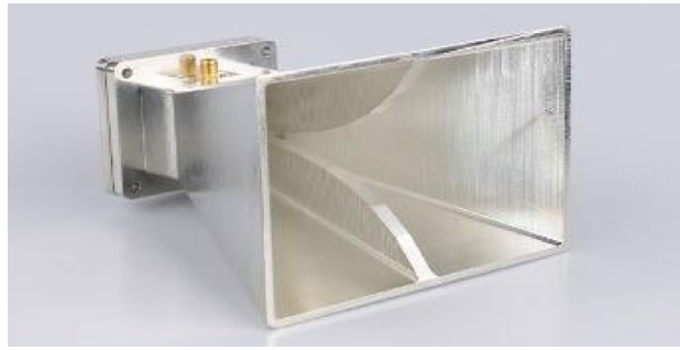
Fig. 10. A fabricated antenna with horizontal polarization.
