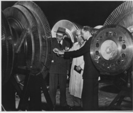
Belgian electrical engineers inspecting the rotor of a 40,000 kilowatt turbine of the General Electric Company in New York City
